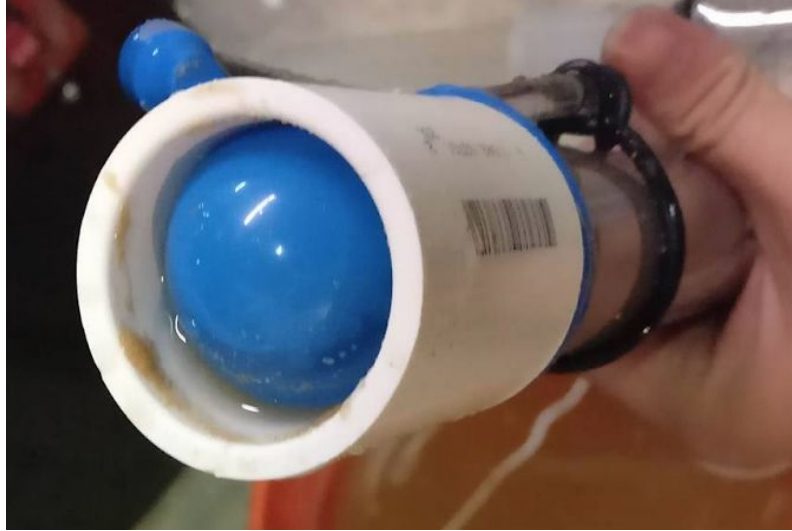
Figure 11. Iteration IV (final) of the Lion Drill: inflatable closing mechanism
